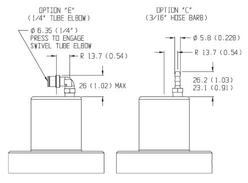
Dimensions in Millimeter (Dimensions in Inches)
