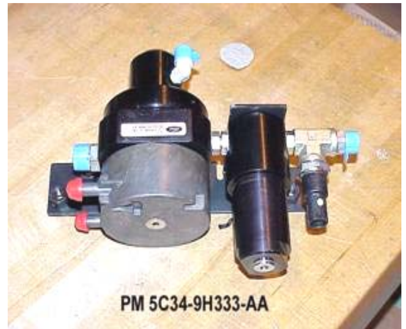
Regulator customized as an assembly with filter, sensor, and fittings
