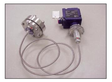
The 330A and 110P are connected via a ten-foot capillary tube. This system was selected to protect the process and operator should an upset occur resulting in extremely high steam temperature or contamination. Due to the versatility we have within the ITT family of Industrial products, we were able to offer the solution entirely in-house. The end customer received a complete package preset and delivered to their facility ready for installation.
