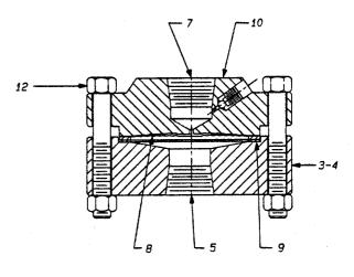
1. Standard diaphragm material is 316L Stainless Steel for seals with lower housing manufactured of CS, S4, S6, SF and SL.
