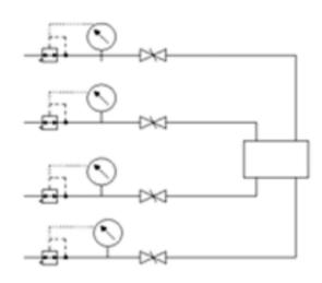
The four GH10 Series Manual Loading Regulators required for this application each have a modified mounting bracket that adapts to a small servo motor. The motors receive a 4-20 mA DC signal from four corresponding pressure transducers. The regulators control the pressure of the four types of gases to the cutting nozzle. A pre-flow gas which is an arc starting gas, a plasma gas which is a cutting gas, a shielding gas which surrounds the arc and a post flow gas.
