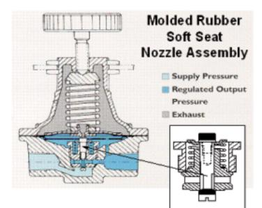
ply air or process media to flow downstream or vent to atmosphere. The top rubber molded seat allows for minimum air consumption under flow conditions.
