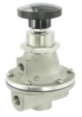
The standard low pressure nozzle assembly is equipped with a metal to metal seating surface. This assembly will allow leakage of the supply pressure to pass by the seat when the nozzle is in the closed position at a rate of 100 cc/minute or less. This keeps the regulator in a dynamic state lessening the pressure drop when there is a demand for flow.
